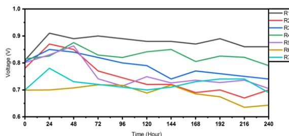
**Figure 4.** Electrical voltage variations in the septage sludge and EM4 Bacteria
