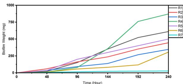
Figure 9. Biofilm weights on the anode
