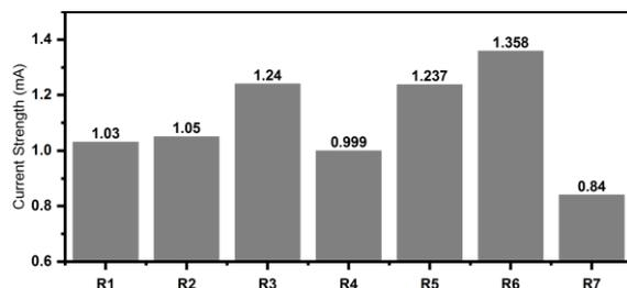
**Figure 3.** Comparison of Electric Current Strength under Different Variations in septage Sludge and EM4
