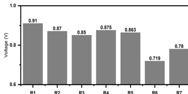
**Figure 5.** Comparison of Electrical Voltage at Different septage Sludge and EM4
