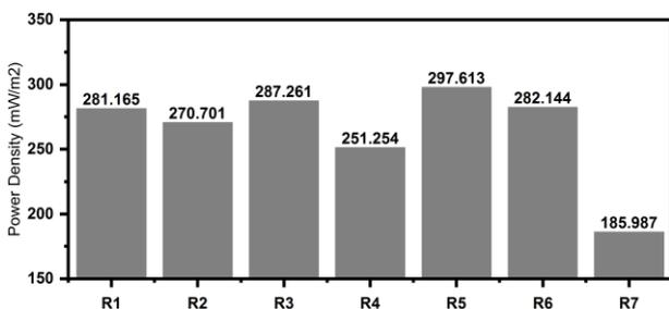
Figure 7. Comparison of power density among septage sludge dan EM4
