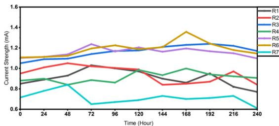
**Figure 2.** Electric current strength of different septage sludge and EM4
