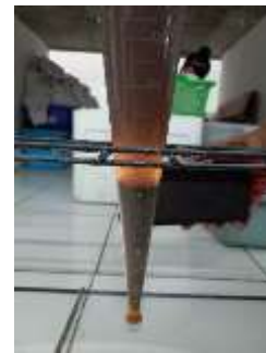
Gambar 5. (a) IPAL Sentra Ikan, (b) Hasil Sampling Lumpur IPAL Sentra Ikan, dan (c) Settleability Test
