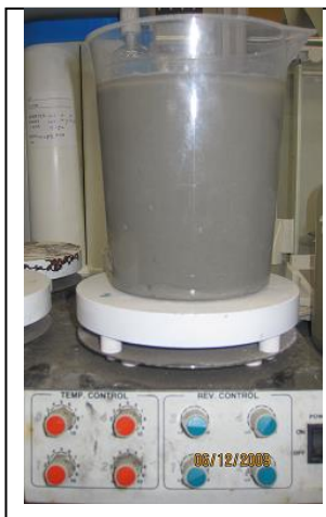
Figure 2. Fly Ash and Distilled Water is Stirred.
