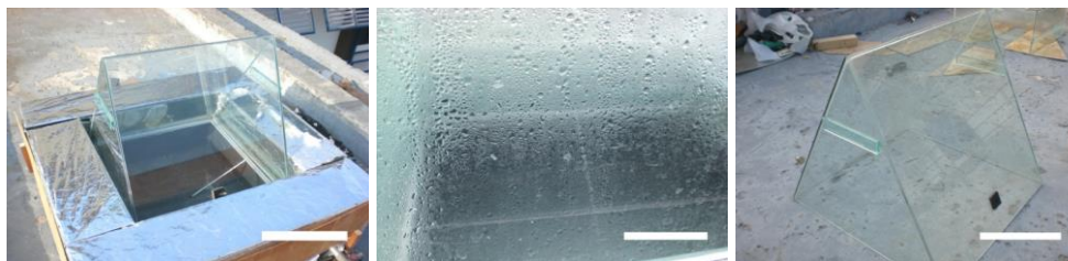
Gambar 5. Distilator Atap Miring
