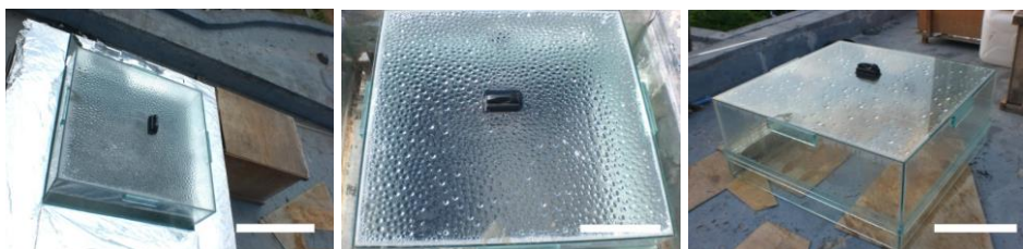
Gambar 6. Distilator Atap Datar
